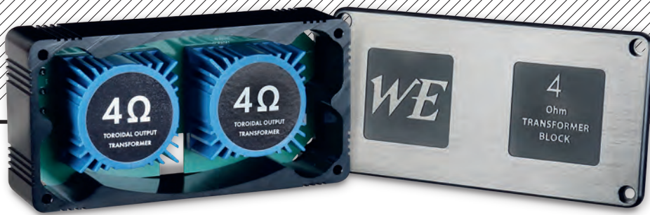
ABOVE: Rather than have multiple secondary windings, and multiple 8ohm, 4ohm, etc, speaker output taps the 91E has interchangeable output transformers specified at the point of ordering
