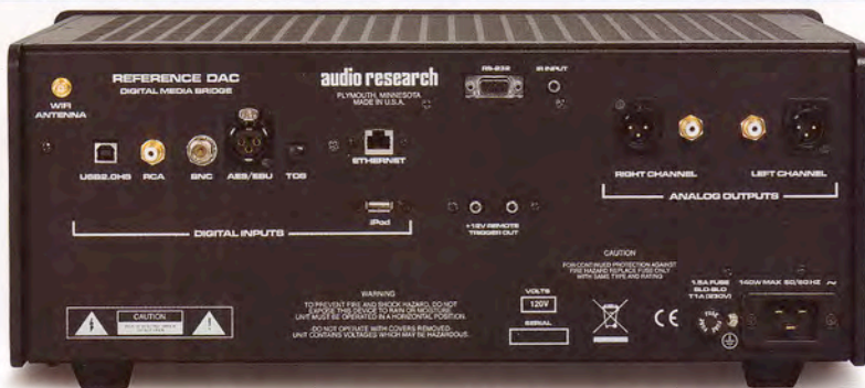
ABOVE: Balanced (XLR) and single-ended (RCA) analogue outputs are joined by USB, three S/PDIF and one AES/EBU digital input plus wired (and wireless) ethernet hubs
