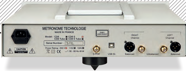
ABOVE: The USB-B and S/PDIF inputs address the same DAC stage as the CD8 Sig's CD section. Analogue outputs include both single-ended (RCA) and balanced (XLR)
